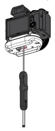
**8** Due to floating design of mounting screw, camera can be adjusted to ensure camera is mostly centered.
