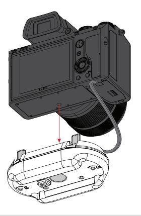
6 Plug in charge cable, routing the wire through the channel to either side of puck. This will depend on where the battery door is located on for your camera.
