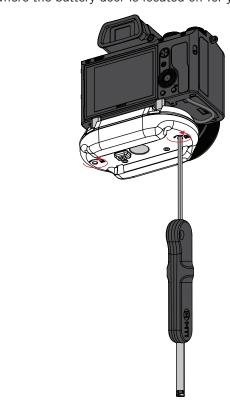
**7** Due to floating design of mounting screw, camera can be adjusted to ensure camera is mostly centered.
