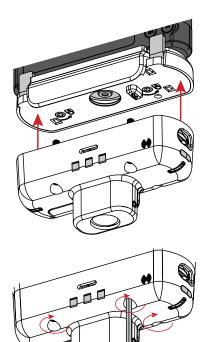
6 Connect the charging cable to the camera. Insert USB-C end of cable into puck until it clicks, indicating it is locked in place.
