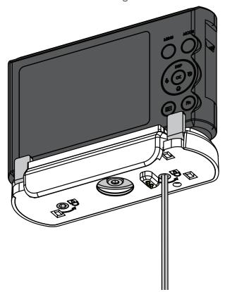
Secure the camera to Shell 1 using the MTI Retail Tool.
