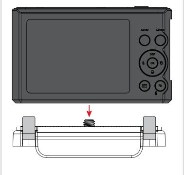
**2** Due to floating design of mounting screw, camera can be adjusted to ensure camera is mostly centered.
