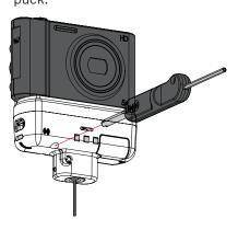
Twist the MTI Retail Tool clockwise 45 degrees and hold it in place.
