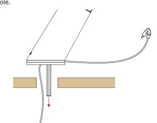
**2** Align bottom plate to slot adapter.
