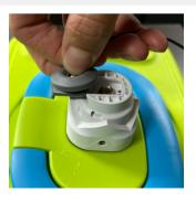
Slide the tether attatchment into the puck to secure the Freedom Micro to the Kids case.
