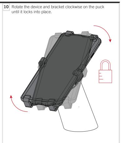
Grab the exposed portion of the puck with your thumb and forefinger. Move the phone back and forth to checking to ensure the bracket locked in place.
