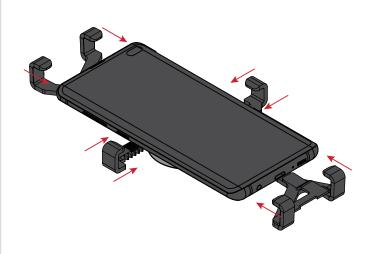
Tighten center locking security screw on the SpeedBracket™ to secure the bracket arms in place around the device. After tightening screws, wiggle the arms to ensure they have fully engaged the lock teeth.
