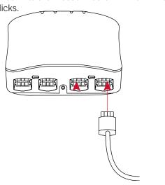
**5a** If using CX Flex<sup>™</sup> insert the USB-C end of the sensor into the CX Flex<sup>™</sup> until it clicks.
