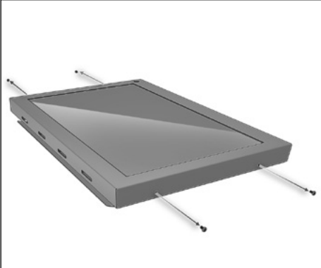
15. Use T-8 Torx Key to remove screws from sides of monitor shroud as shown.
